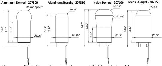
All covers are fitted with an M5 countersunk screw, sub-flush from the top of the cover.
